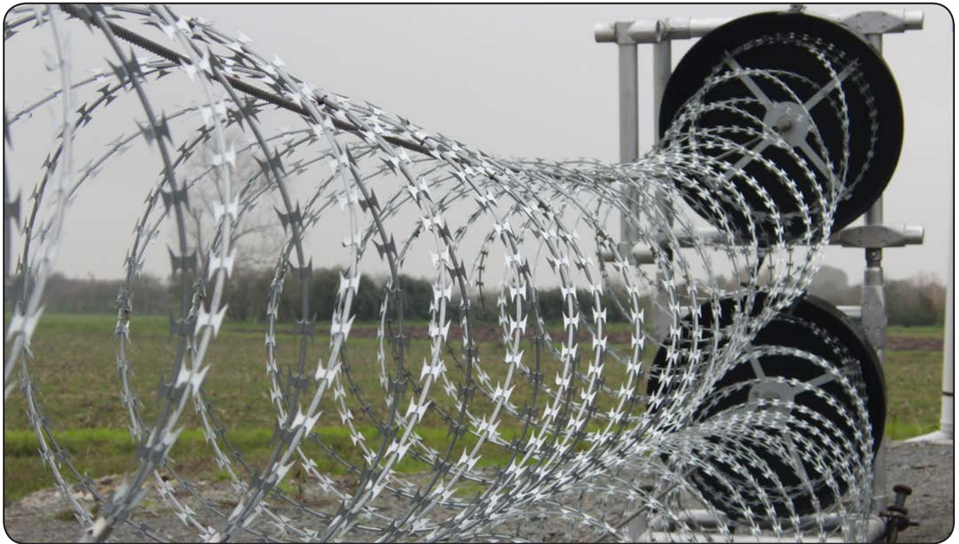
The system when open. The capsule is equipped with 10 metres of razor wire.
